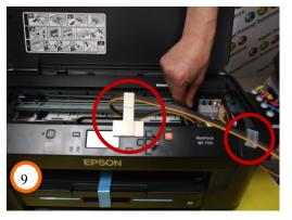
10) Place the adhesive clip and the pipes (photo 9).
