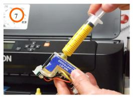
8) Insert completely the syringe tip in a cartridge valve and aspire until the syringe is full of ink. You can return the ink that is accumulate in the syringe in the tank of the corresponding color. Repeat the operation for all the colors. (Photo 7)
