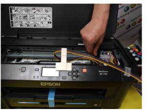
11) For the right functioning the pipe should not ridde the the trolley race. To make shure that it moves correctly we raccommend to move manually the trolley to the right and to the left (photo 10-11). In this way you can adjust the pipe length so that, during the movement will always remain well stretched out and do not tuck into itself.
