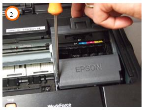
3) Manually move the printer trolley in the cartridges change area, gently remove the trolley cover levering with a flat-blade screwdriver. Photo 2
