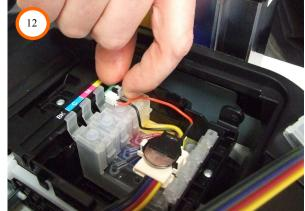
13) When you see the message of empty cartridge it will be necessary bring the machine in cartridge change position following the display instructions, it will not be necessary remove the cartridges, you just have to press the reset button for 10 seconds. Photo 12
