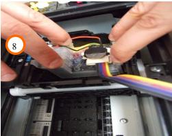
9)Place the cartridges in the print trolley and press the block untill you hear the hooking click. photo 8
