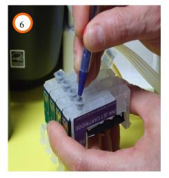
7) Reverse the cartridge group. With a pen tip pierce the plastic operulum that protects the valves (Photo 6).
