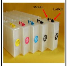
1– In the cartridges back side there are two holes the larger one is for refill, the smaller one is for the air. When you completed the recharge you must let the air hole open to allow the correct working of the printer.
